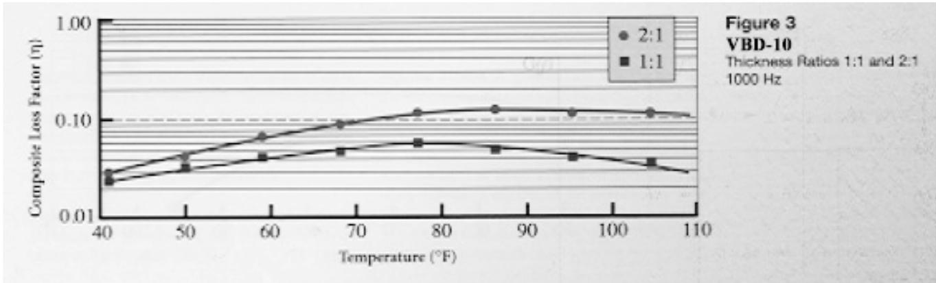
Though there exists a loss factor of the damping material itself, generally a loss factor refers to the system of the damping material on a base layer whose vibrations are to be damped.
