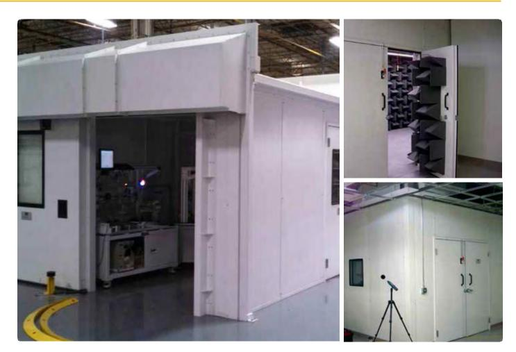
INC PANL-WALL® TEST & MEASUREMENT CHAMBERS provide a controlled acoustical environment to perform accurate, repeatable product testing. Our systems provide high acoustic isolation from ambient environment and low interior noise level.
