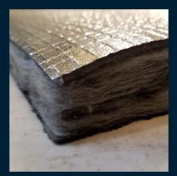
ANC-CB22 combines a flexible 1 lb/sq ft foil faced loaded vinyl noise barrier with a 1" fiberglass decoupler to enhance its noise reduction properties.
