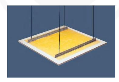
Barricade™ Ceiling Clouds are perfect for the reduction of sound in ceiling areas. They are suspended horizontally with eye hooks (for panels up to 4'x 4') or T-grid attachment. The T-grid may be attached in the field or at the factory before shipment for your convenience.
