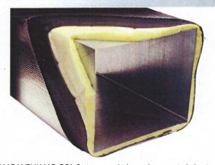
ANC-WBV/ANC-QFA-3 is a multi-layered acoustical lagging designed to reduce noise that radiates thru the walls of ductvork or piping. Cutaway view shows the quilted fiberglass decoupler, the loaded vinyl noise barrier and the outer reinforced foil jacket.
