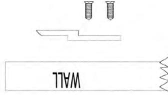
4. Slide the EC-1 brackets on the panels onto the EC-2 / EC-4 bars on the wall.
