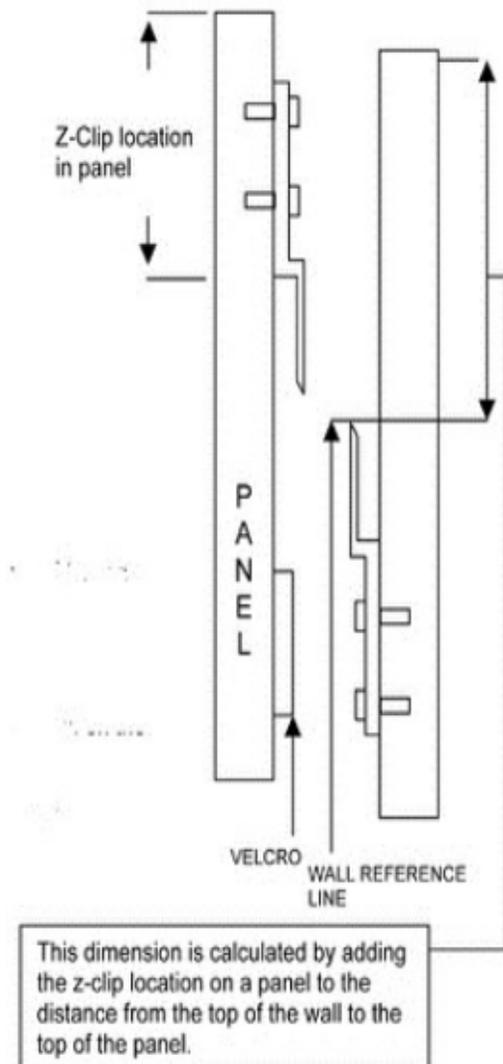
**Another mounting option for Acoustical wall panels that must be removable is Z-Clips and Velcro dots:**
