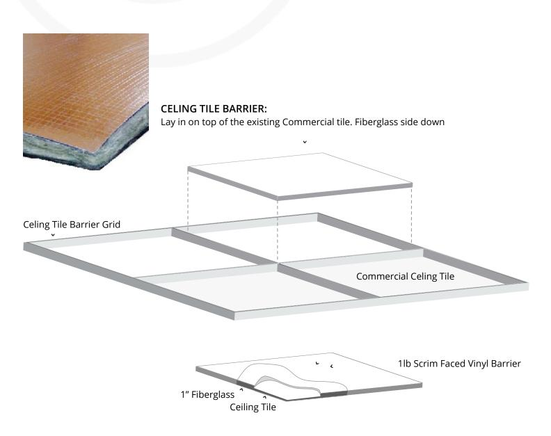
BLOCK TRANSMISSION OF SOUND THROUGH FLOOR AND CELLINGS.
