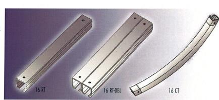
\* 16 CT curved piece has flared ends, the same dimensions as a connector piece, and will accept straight track pieces fitted into its ends. Once assembled, it functions as a continuous piece of track. Curved connectors are available with mounting hardware for floor, suspended, wall, ceiling mounted or HD systems.
