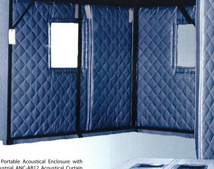
This three-sided Portable Acoustical Enclosure with roof utilizing Industrial ANC-AB12 Acoustical Curtain Panels was designed for approximately 20 dB (A) noise reduction. The entire enclosure is mounted on casters to allow for complete accessibility to equipment. Clear vinyl view windows offer visibility.
