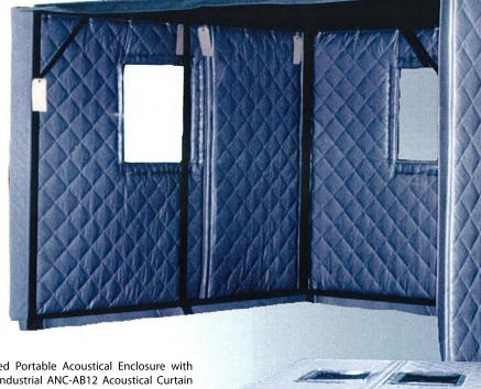
This three-sided Portable Acoustical Enclosure with roof utilizing Industrial ANC-AB12 Acoustical Curtain Panels was designed for approximately 20 dB (A) noise reduction. The entire enclosure is mounted on casters to allow for complete accessibility to equipment. Clear vinyl view windows offer visibility.
