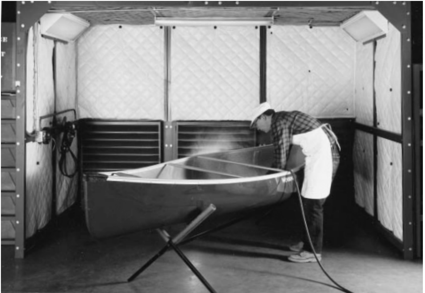
All Noise Control ANC-ANC-QFA-10 (White) reduces noise levels inside and around this environment control booth.
