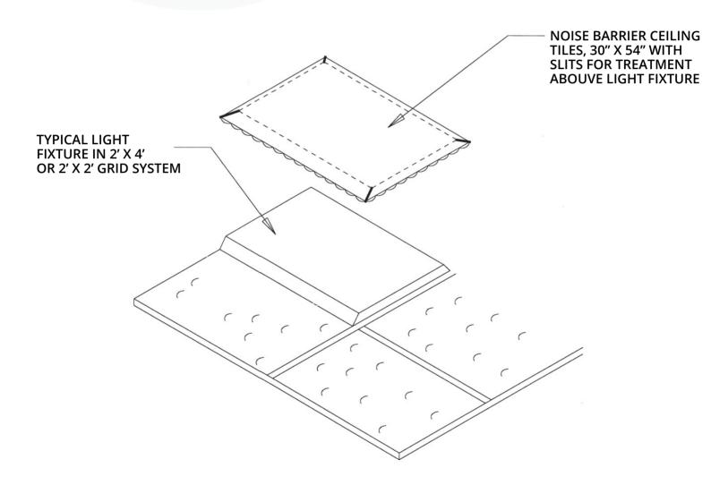
TREATMENT ABOVE CEILING SYSTEM FOR IMPROVING TRANSMISSION LOSS ABILITY
