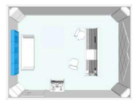
The most common placement for diffusers is at the rear of the room where direct sound coming from the monitors can pose problems by creating powerful reflections. For great results, most designers will gang several F Diffusers together that will span the entire work area behind the listening position.
