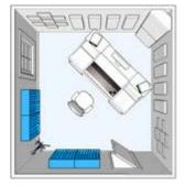
In smaller rooms, the F Diffuser can add a sense of space and air in by spreading sound energy around the room. The variable slats allow you to redirect the energy away from the primary listening space and use the natural room boundaries to diffuse the high frequency energy.
