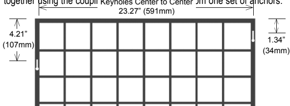
Keyhole locations when viewing the RD Diffuser from the front with keyholes on the back side: Horizontal measurements between anchors is 23.27" or 591mm center to center.
