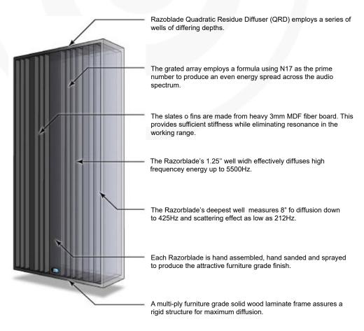
The Razorblade<sup>™</sup> is a 24" x 48" x 8" (61cm x 122cm x 20.3cm) quadratic residue diffuser (QRD) that will effectively break up standing waves and directional reflections to provide a sense of air and increased space in any room. Ideally suited for recording studios, theaters and critical listening environments, the Razorblade features a series of 17 wells of varying depth that combine to effectively scatter frequencies as low as 400Hz.
