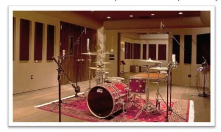
good the microphone, preamp or recording system, unless the acoustics are balanced, your recordings will translate well when played back on other systems. Hard surfaces such as gypsum walls, windows and hardwood floors cause primary reflections which make placing instruments in the stereo field difficult. Secondary reflections introduce flutter echo and a reverb trail which interferes
