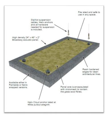
of the wrist. The clever Helix anchor twists into the back of the high-density glass wool panel and is rated at 45lbs pull-out strength. A generous amount of suspension tie wire is included. Everything you need is in the box.
