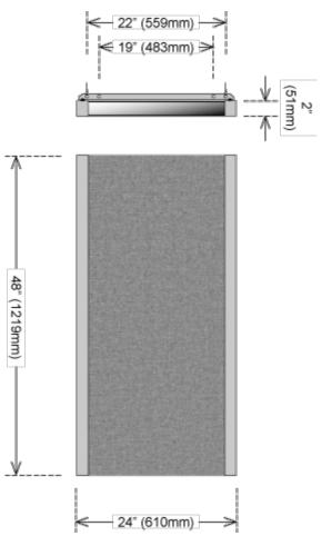
The Prima Stratus is an acoustic cloud system designed to create large acoustic ceilings by linking multiple units together with a rigid frame.
