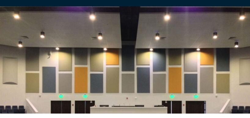
Acoustical Wall panels are sound absorbing panels that can mount directly to walls or ceilings through a variety of adhesives, impaling clips, hook & loop fasters etc. They are designed to stop noise control issues with their powerful sound absorbing acoustical materials. They are frequently used in offices as they not only prevent noise pollution but increase speech intelligibility by reducing reverberation and echoes
