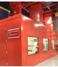
INC PANEL-WALL® product line consists of pre-engineered, modular acoustical panels and components that can be configured and assembled into a wide variety of structures. Panel-Wall is particularly suited for applications requiring a high degree of noise reduction of up to 40 decibels or more.
