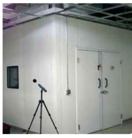
**INC PANEL-WALL® TEST & MEASUREMENT CHAMBERS** provide a controlled acoustical environment to perform accurate, repeatable product testing. Our systems provide high acoustic isolation from ambient environment and low interior noise level.
