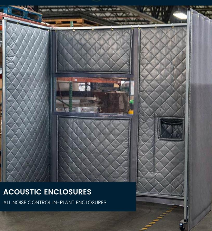
Industrial In-plant Enclosures are available as complete, Partial, or portable enclosures. Enclosure options include sliding dor panels, view windows, strip doors, air intake and exhaust ventilation baffles, partial or full roof panel systems, and corner strips among many other features.
