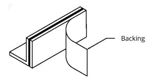
1 Attach the base angles to the "Z"-bars. level and adjust as necessary. In the vicinity of the velcro push the diffuser firmly onto the wall.
